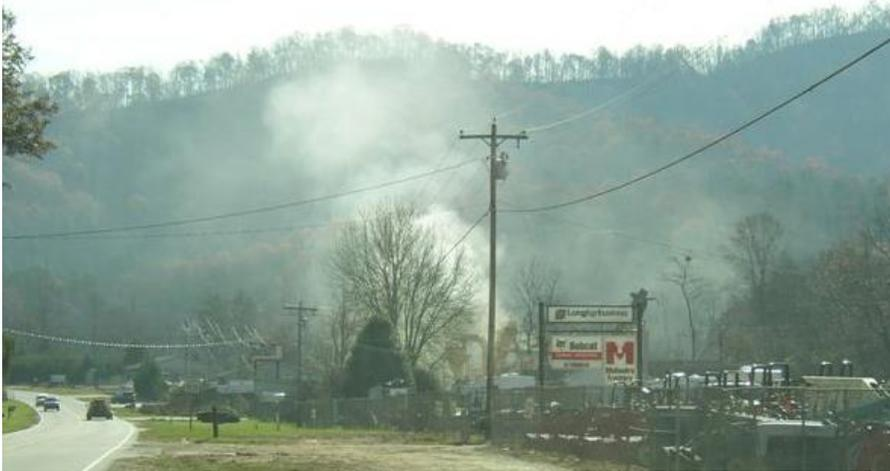
Fugitive emissions are pollutants not emitted from the stack but released to the atmosphere. Based on the annual consumption of asphalt cement, one can calculate the asphalt vapor fugitive emissions from any plant. Asphalt cement typically comprises 5% (0.05) of the total hot mix plant production. Fugitive air emissions equal 1.07% (0.0107) of the consumed asphalt cement.<sup>1</sup>
